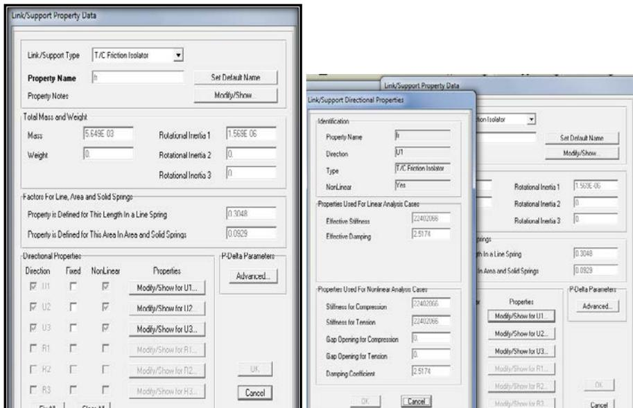
Fig(7) Link/support property data] ,and Link/support property data for  $U_1$
