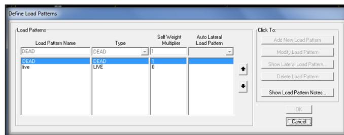
Fig(10) Load pattern Assignment
