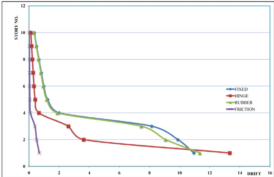
Fig.(16) Hybrid's drift
